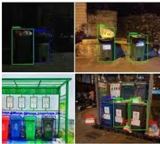
SMART bins – bin overflow monitoring through computer vision analytics
